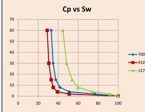
The same curves are shown after a conversion to height using parameters appropriate for the reservoir. For a sample reservoir, three capillary pressure curves at their reference permeabilities are shown, in terms of Cp vs Sw.
