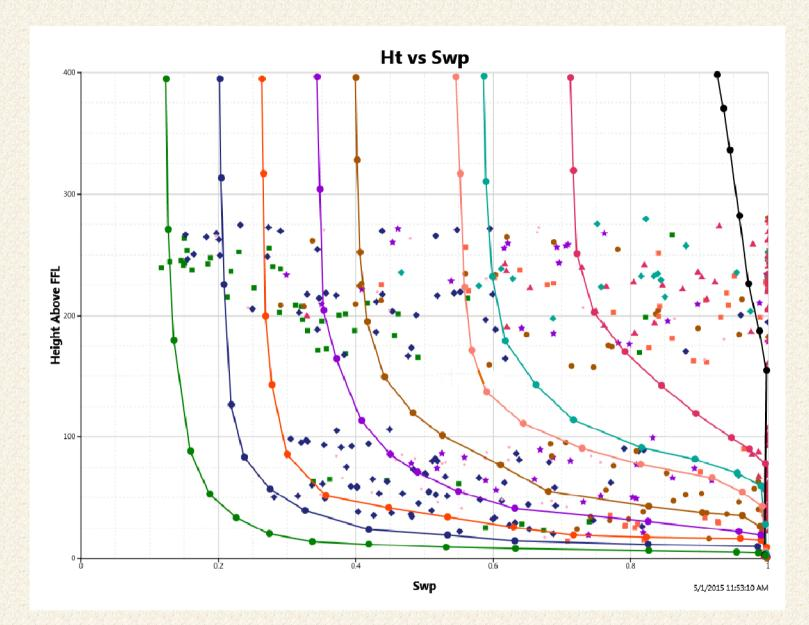
This process is continued until all data are posted and curves are fitted. A final very low-permeability curve (black) is drawn to provide a lower bound for the set of pseudo-capillary pressure curves.
