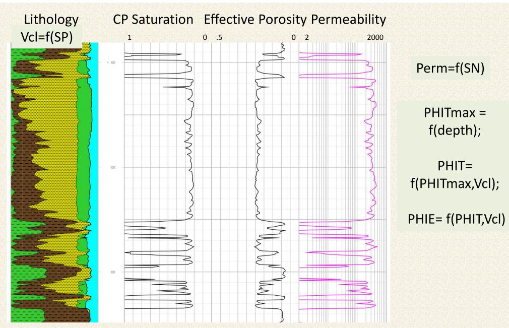
In this example of a 1950's well with an old e-log, reservoir properties were derived from the SP, SN, and local knowledge. The SwCP was calculated from a set of core-derived pseudo-Cp curves.
