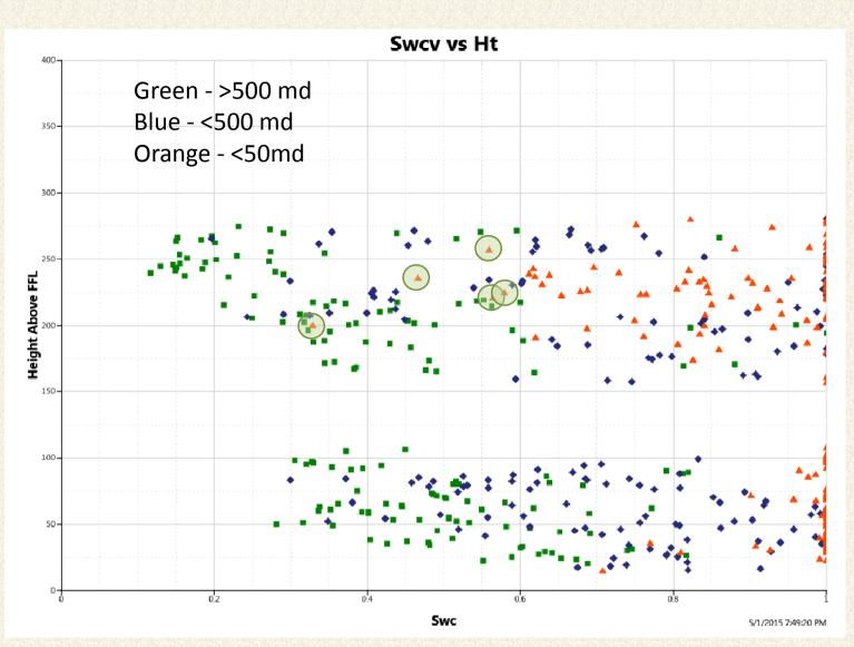
In general, the higher permeability samples have lower Sw and lowpermeability samples have higher Sw. The spread of high-permeability data from left to right shows the effects of partial depletion in the reservoir. Some of the very low permeability samples (orange) have anomalously low Sw; they likely represent damaged samples or inaccurate data.
