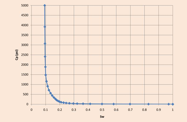
Above a certain pressure, very little additional water is displaced and the curve become asymptotic. The minimum Sw reached is equivalent to the irreducible Sw at that permeability.
