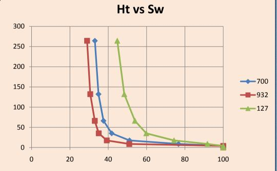
Capillary pressure curves have a characteristic shape as shown above. They also have a characteristic ordering, in which higher permeability samples have a lower Swirr than lower permeability samples. The entry pressure (and therefore entry height) is also higher for low-perm rocks.
